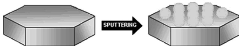
Figure 1. Representation of the deposit of the CuNPs on the plane (001) crystal of the IC.
